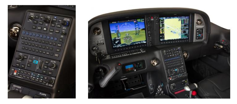
**ABOVE, LEFT:** The all-new keypad in the Perspective+ cockpit has several brand-new features. Note the laterally arrayed number pad for entering frequencies and transponder codes. Near the bottom of the pad is the autopilot controller, and toward the top center is the brand-new home key for easy keypad nav.
