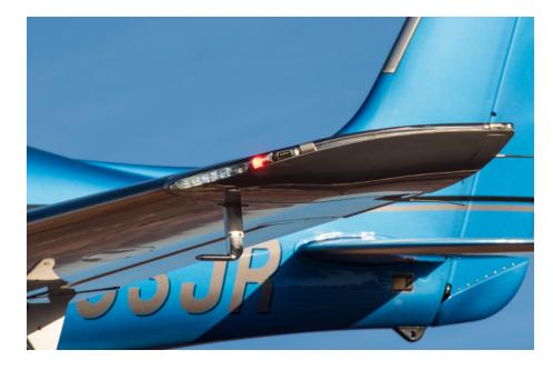
The new Spectra wingtip lighting system is many things at once—a recognition system, bright nav lights, strobes and landing lights all in one. The bright and flexible all-LED system is anchored by a long light rope that can act as a strobe, a pulse light or path lighting.
