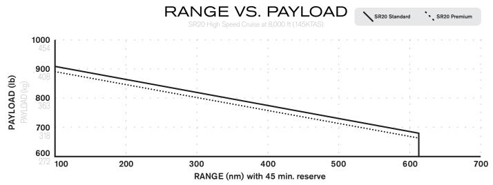
+1 lb (.45kg) Payload or Equipment = -2.2 NM 65% to 55% PWR = +8% Range
